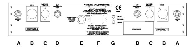
A) LIMITER IN. This is a balanced input that allows you to get a signal straight into the opto-limiter without going through the mic pre and EQ. As soon as you insert a plug into this jack, it breaks the normal signal path TIP = +, hot or positive going signal from the EQ. The pin-out is as follows:
